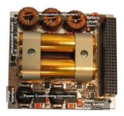
This type of supply is capable of providing power directly from the solar panels in the event that, after some time in space, the battery no longer holds its charge. This will permit sunlight-only operation of the spacecraft after a battery failure; this was an early mission requirement.
