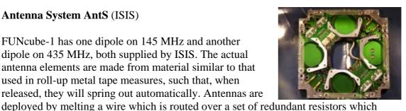
can be heated on command. When the wire melts it releases the lid allowing the antenna to deploy. The antennas will be deployed (one element at a time) approximately 10 minutes after ejection from the ISIPOD; this is to make sure that we are at a sufficient distance from the other payloads so we don't hit anything.
